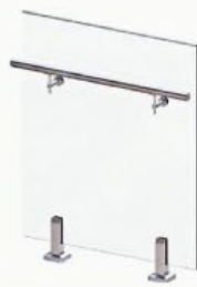
HLS-002 Class base 50x50xH200mm 10-12mm Glass Maximun separation:1200mm
