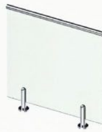
HLS-003 Class base \varnothing 50xH180mm 10-14mm Glass Maximun separation:1200mm
