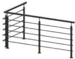
HLS-021 H950mm-Ø38.1mm Ø12mm Horizontal bar or tube Maximum separation:1200mm
