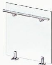
HLS-007 Class base 50*50*H160mm 10-12mm Glass Maximun separation:1200mm
