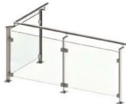
HLS-016 H950mm-45*45mm (arc bottom) 8-11mm Glass Maximu separation: 1200mm
