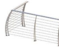
HLS-22 H1200mm-8mm SS Flat bar Middle post and 15mm SS Flat bar End post SS Cable ø8mm Maximum separation:1200mm
