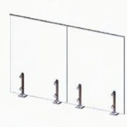
HLS-001 Class base H15x65mm 12-18mm Glass Maximun separation:1200mm
