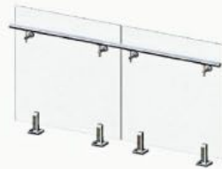
HLS-006 Class base 50x50*H200mm 12-18mm Glass Maximun separation:1200mm
