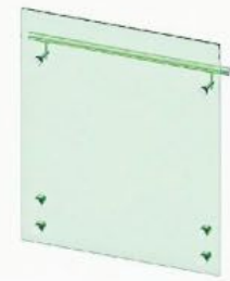
HLS-011 Glass Fastener \varnothing 50mm 12-18 mm Glass Maximun separation:1200m
